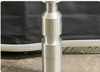
Long connector pin + M18 collar (≈90)
